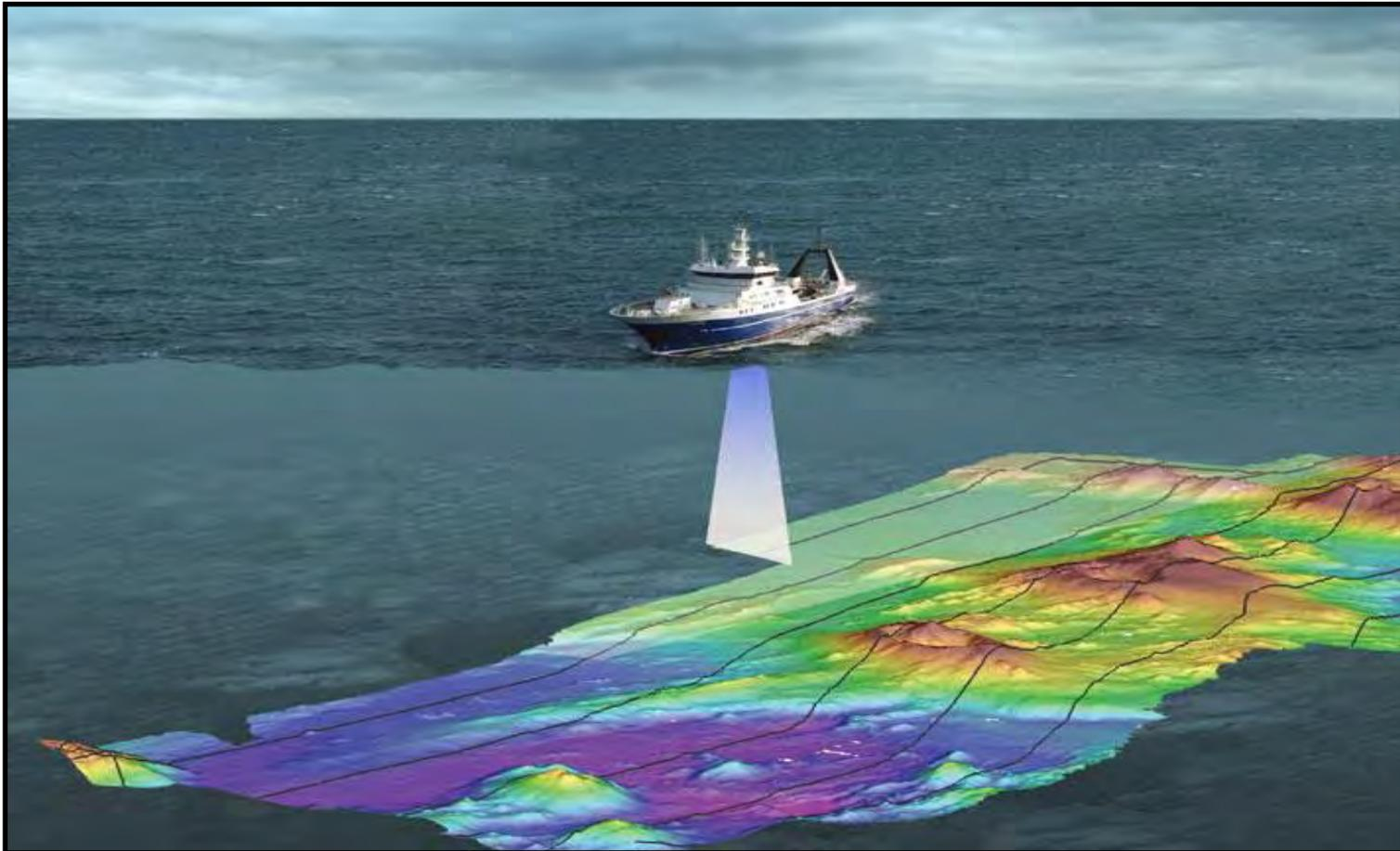
Seabed mapping systems accurately chart depth, topography, slope angles and seabed type
