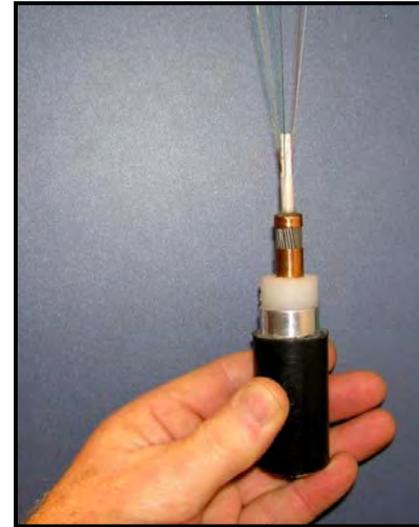
Deep-sea cable, (black) sectioned to show internal construction; fine strands at top are optical fibres used to transmit data
