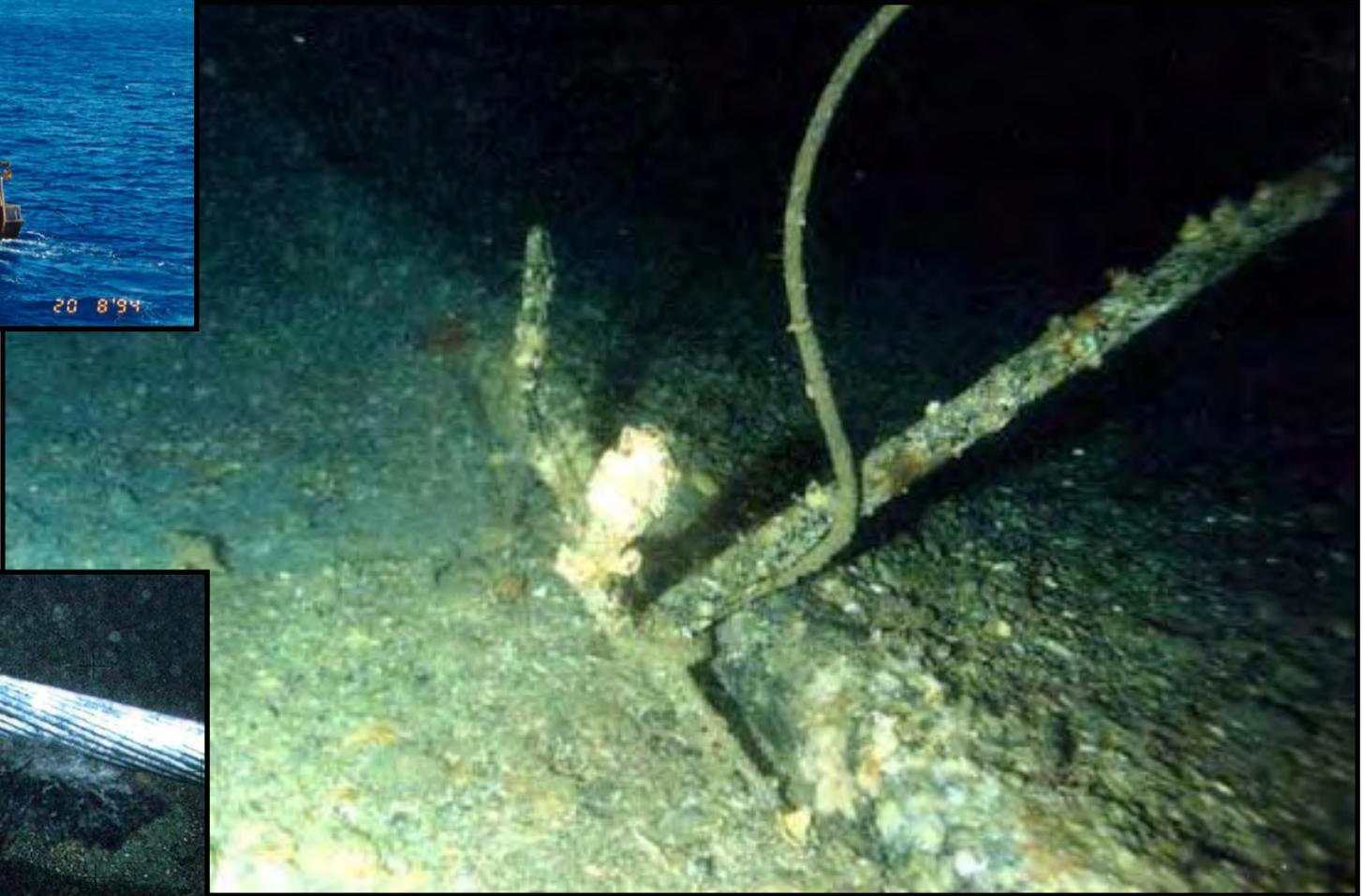
Cable snagged and moved by trawl gear
