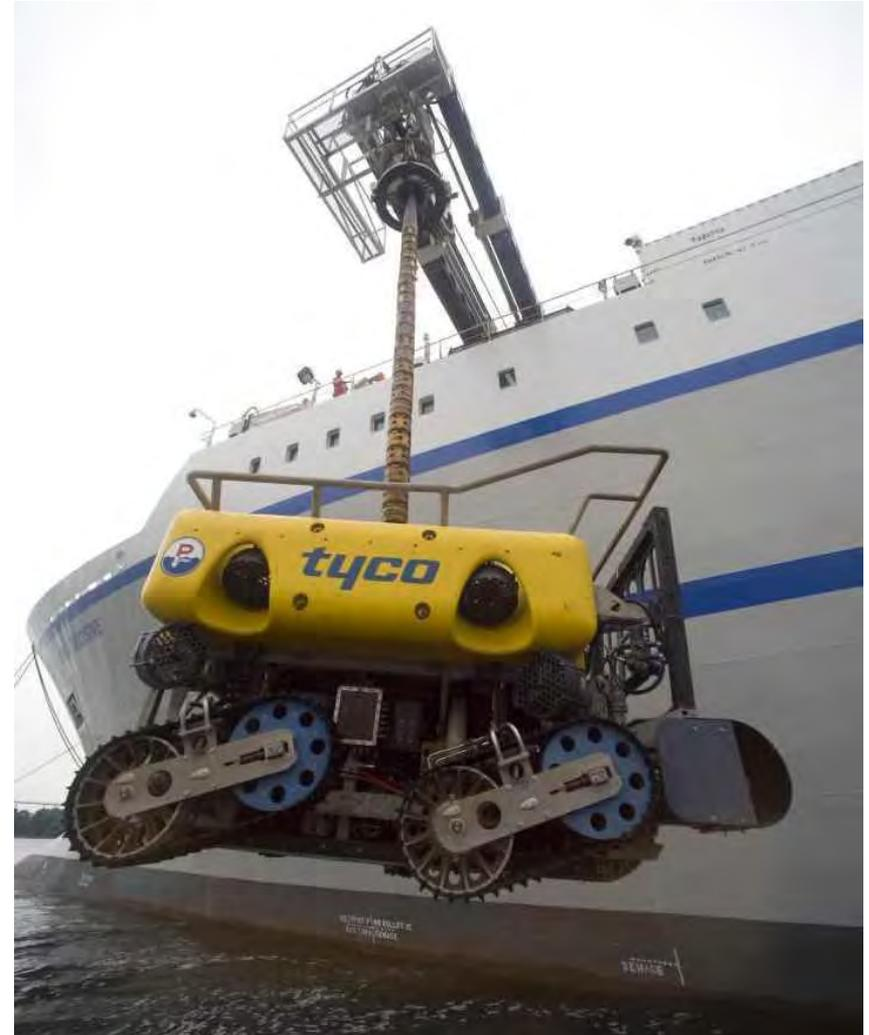
ROV used for cable inspection, recovery and burial
