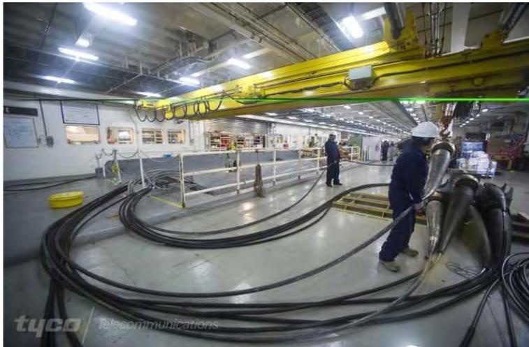
Cable and repeaters inside a cable ship
