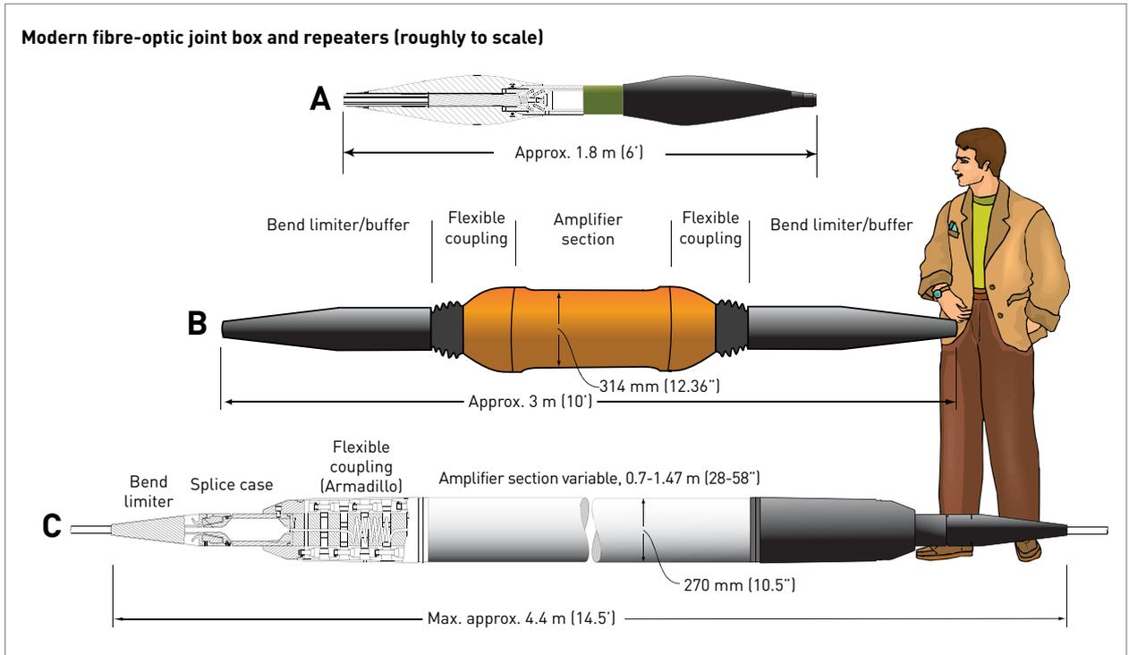
**Figure 2.5: Representative repeaters from different manufacturers. The housings can accommodate as many as eight individual regenerators, or more recently, optical amplifiers.** *Source: Lonnie Hagadorn.*
