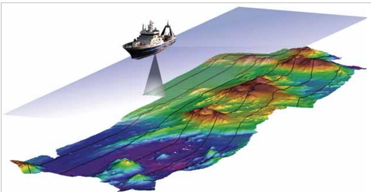
**Figure 3.1: 'Mowing the lawn': a survey ship, equipped with a multibeam mapping system and guided by satellite navigation, charts the seabed to provide total coverage with depth soundings along a swath of seabed that can be 20 km wide.** Source: NIWA.
