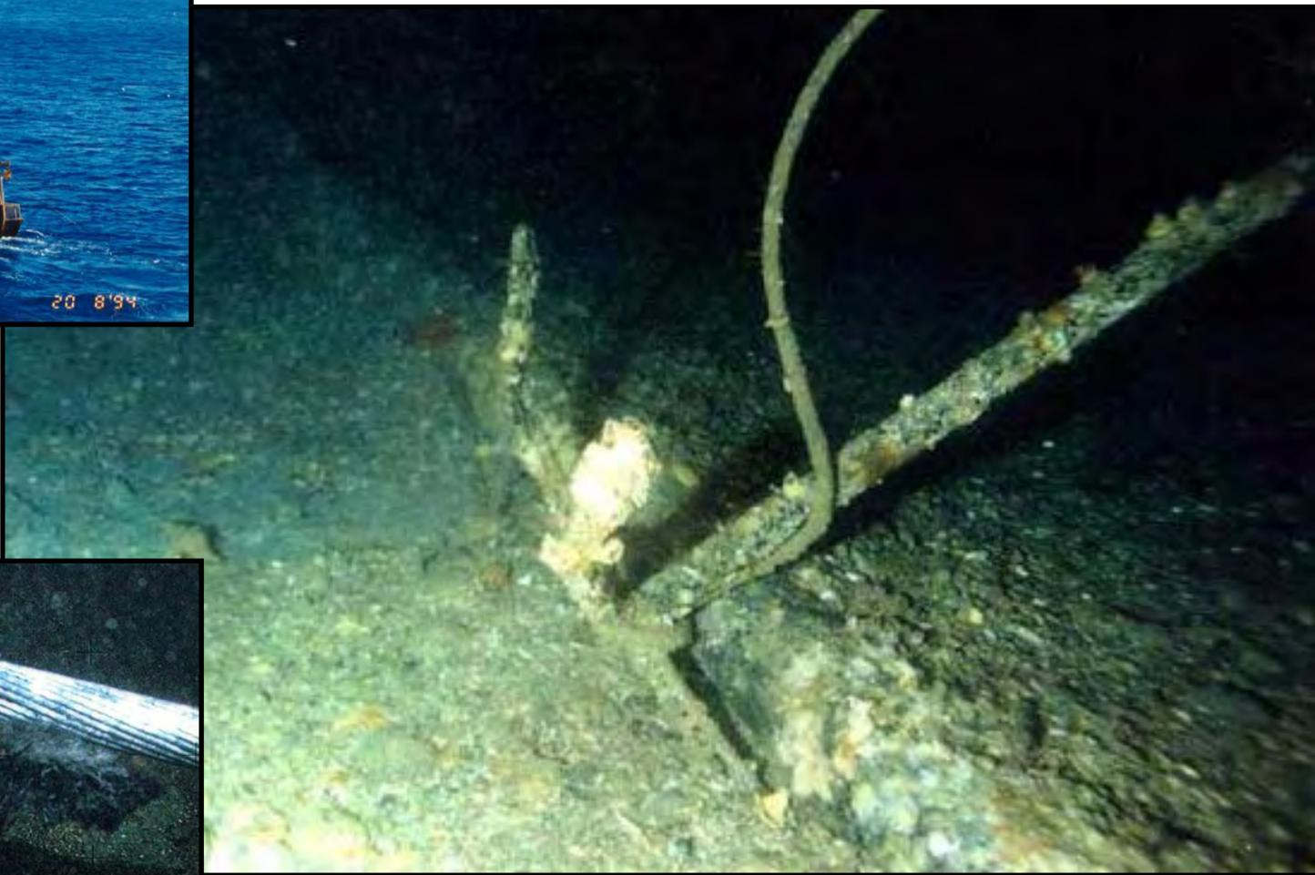
Cable snagged and moved by trawl gear
