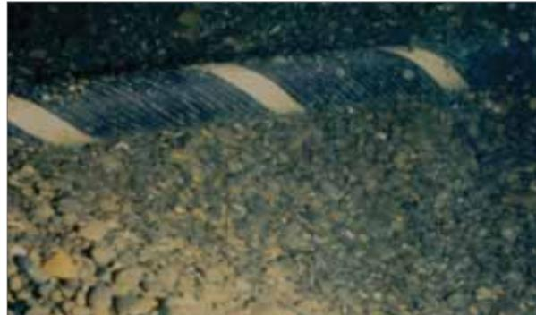
**Figure 3.6: Image of a surface-laid cable taken during a post-lay inspection by an ROV. This image reveals the cable in the throes of burial by mobile gravel.** *Source: Transpower New Zealand and Seaworks.*
