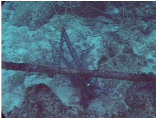
Figure 4. – Galvanized boat anchor found fouled on the cable.
